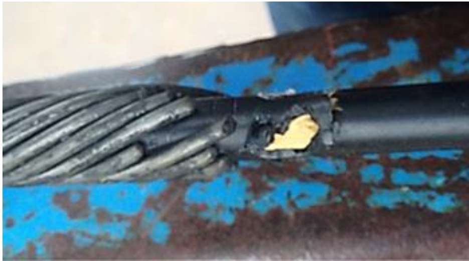
ADSS damaged by electric field
