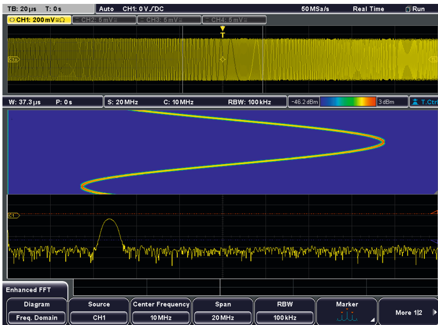
Test signal from three different perspectives: time domain (top), spectrogram (center) and frequency domain (bottom).
