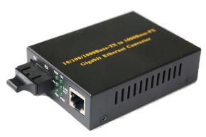
AX-1000MM850D-550/AX-1000SM1310D-20/AX-1000SM1310D-2 complies with IEEE802.3, IEEE802.3u, IEEE802.3z and IEEE802.3ab standards. Presently it supports two types of media network connections: 10Base-T/100Base-TX/100Base-T and 1000Base-SX/LX, inter-converting electrical signals of 10Base-T/100Base-TX/1000Base-T twisted pairs with optical signals of 1000Base-SX/LX.
