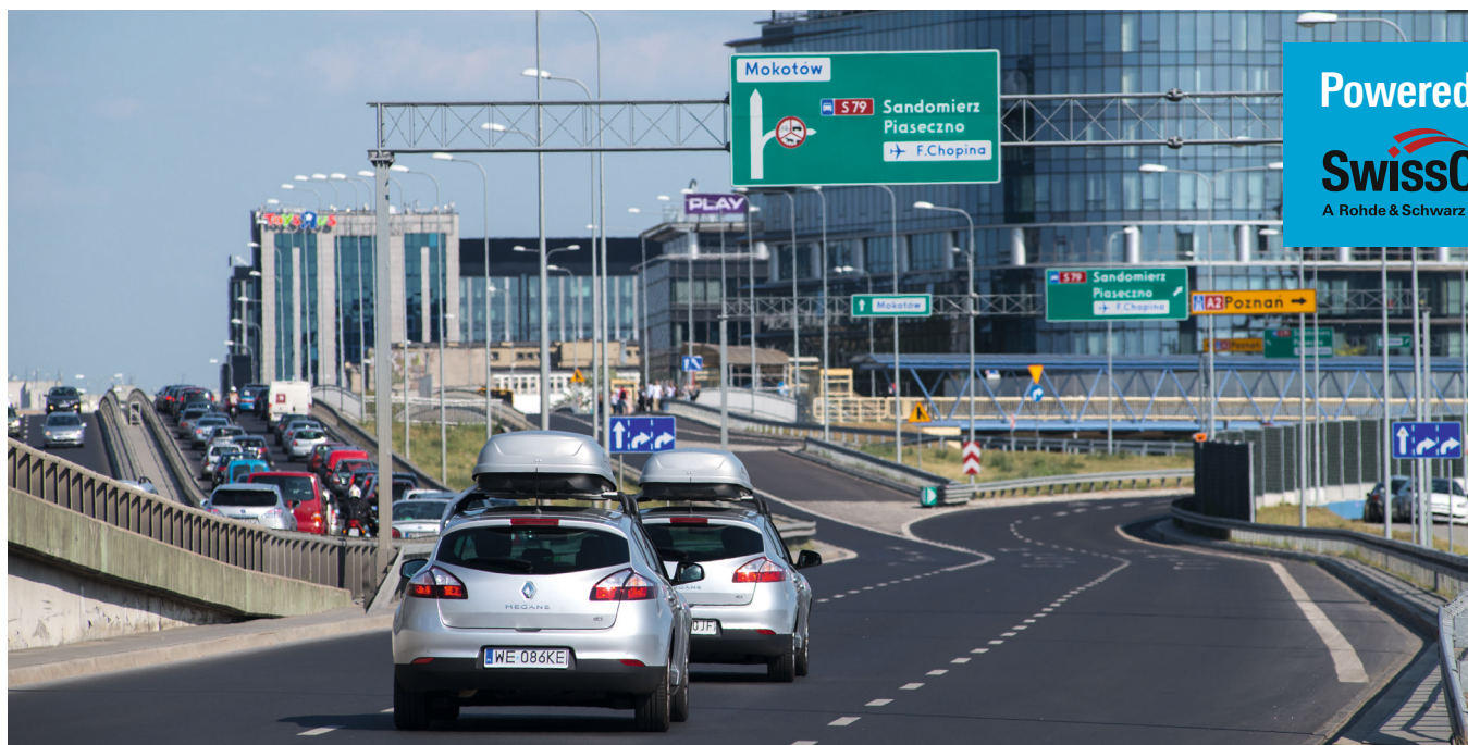
Two of six Systemics-PAB drive test cars with the Benchmarker II testing solution installed in the trunk and the vehicle roof box (VRB), which hosts the devices, on the roof.
