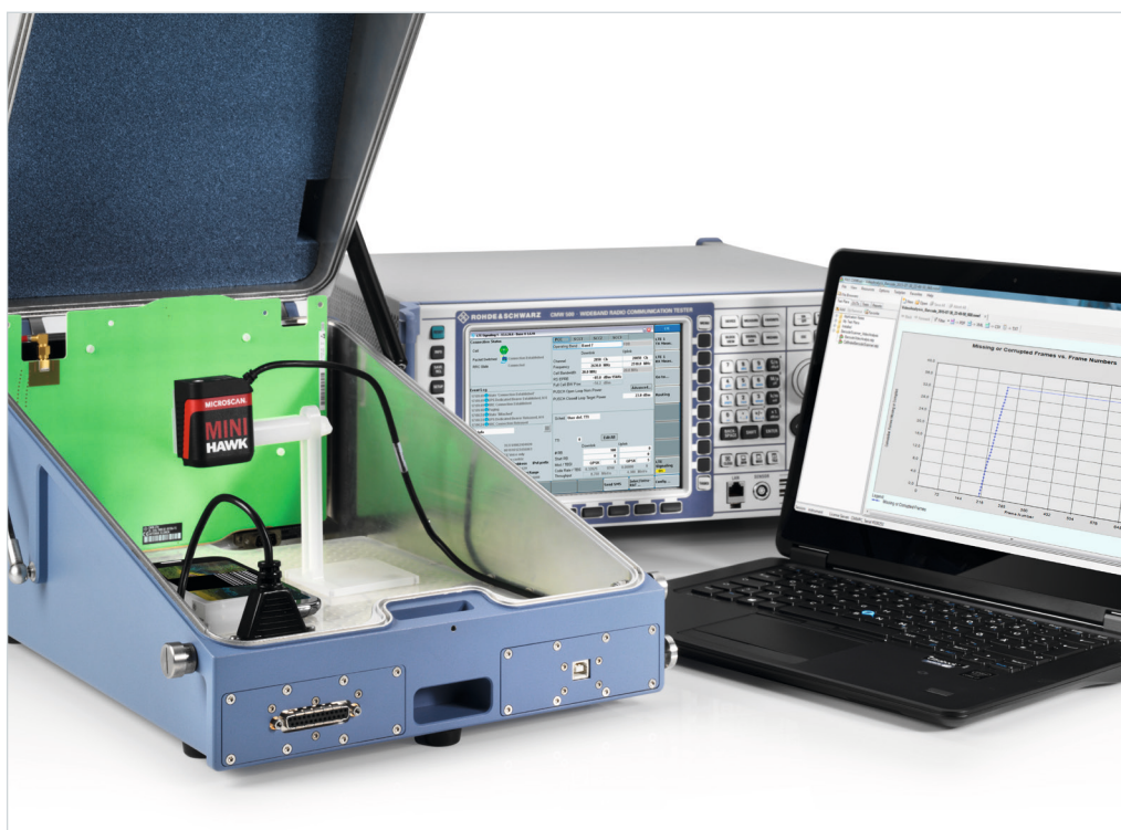
R&S®CMWrun – over-the-air (embedded barcode) video analysis based on R&S®CMW-Z17/R&S®CMW-KT104.
