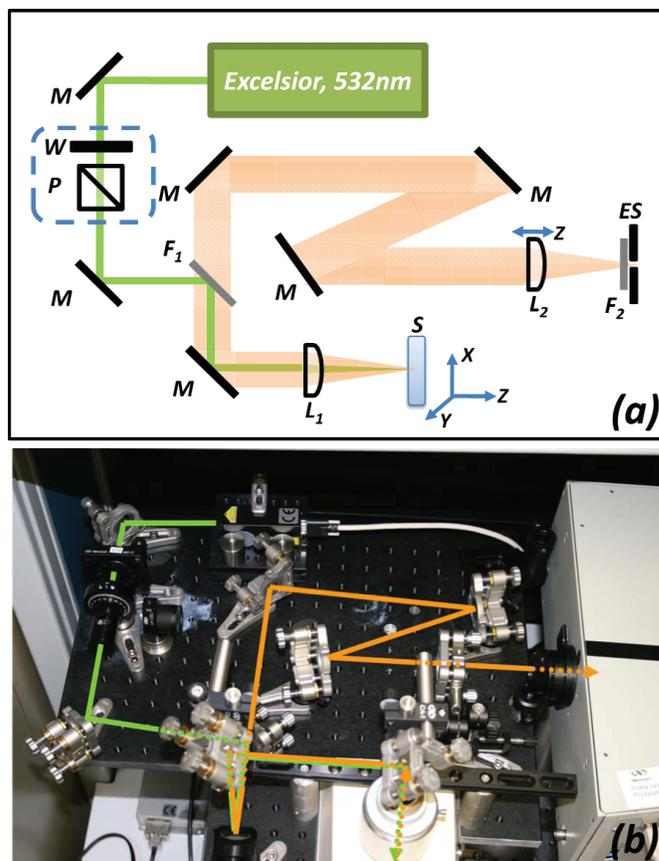
Figure 1. (a) A diagram shows the principle of the experimental setup. M: mirror, W: waveplate, P: polarizer, S: sample,  $F_1$ : 45° beamsplitter,  $F_2$ : long wave pass filter,  $L_1$ : objective or lens,  $L_2$ : condenser lens, ES: entrance slit of the spectrometer. The dashed circle marks the attenuator. (b) Photograph of the Raman Microspectrometer setup in the Newport TAC. The laser is shown in green, while the Raman scattered field is shown in orange.
