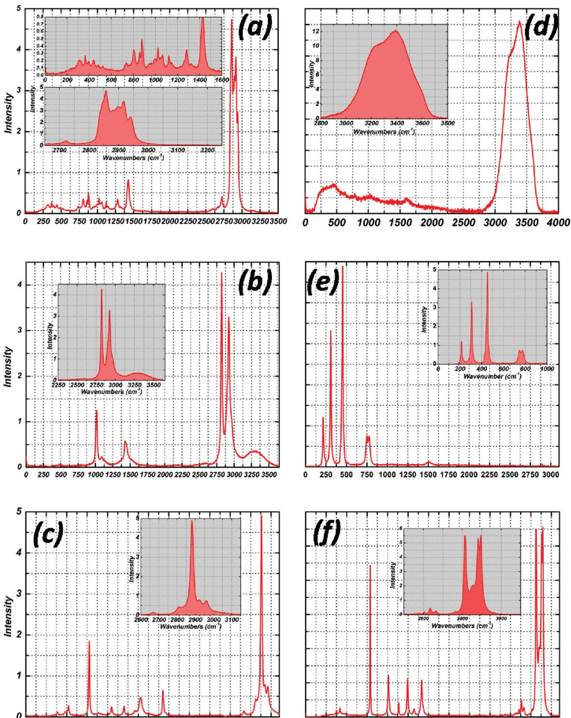
Figure 2. Raman spectra of *n*-hexane (a), methanol (b), acetone (c), water (d), carbon tetrachloride (e), cyclohexane (f). The inset of each spectrum shows the region where the peaks are most congested.
