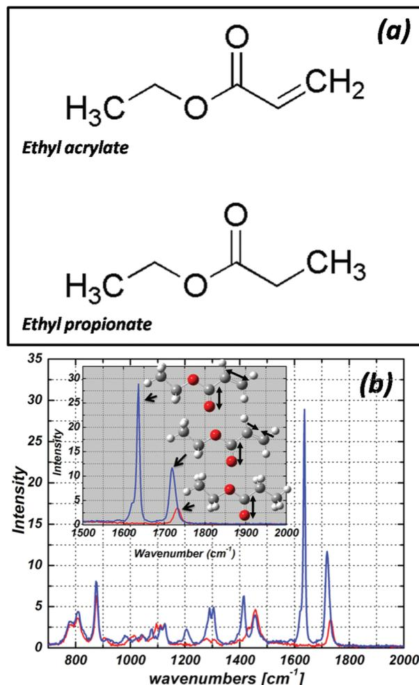
Figure 3. (a) The chemical structures of ethyl acrylate and ethyl propionate. (b) The Raman spectra of ethyl acrylate and ethyl propionate in  $\text{CCl}_4$ . Blue/red traces are for ethyl acrylate/propionate solution, respectively. The spectra in the  $1600\text{ cm}^{-1}$  region are shown in the inset where the dominant displacements of the normal modes are also demonstrated.
