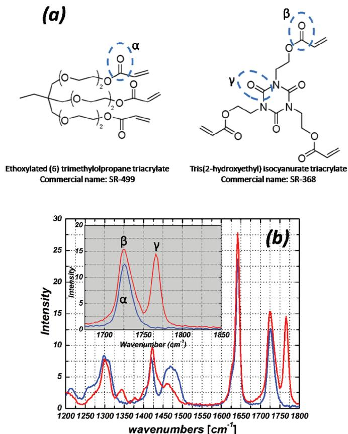
Figure 4. (a) Molecular structures of SR-499 and SR-368. Also shown are the carbonyl groups which contribute to different vibrational modes. (b) Raman spectra of SR-499 and SR-368. Inset: the 1700  $\text{cm}^{-1}$  region is magnified to show different vibrational modes of the molecules.
