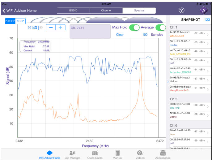
Spectral view shows interference within a channel
